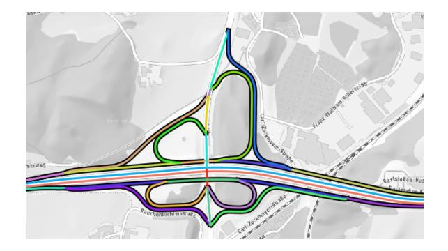
Modelling of a complex motorway junction with several slip roads as sections Example: Junction A1 Westautobahn with B158/B150 at Salzburg North
