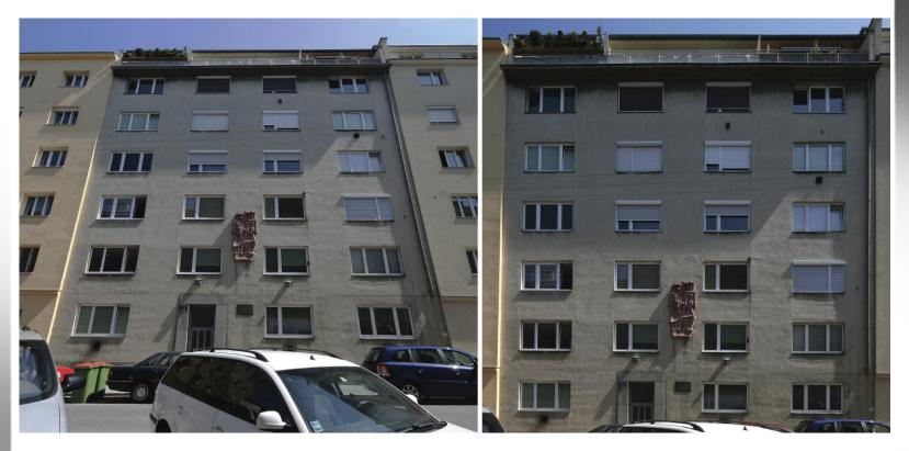
Orthographic facade images were generated using a Tilt-Shift lens
